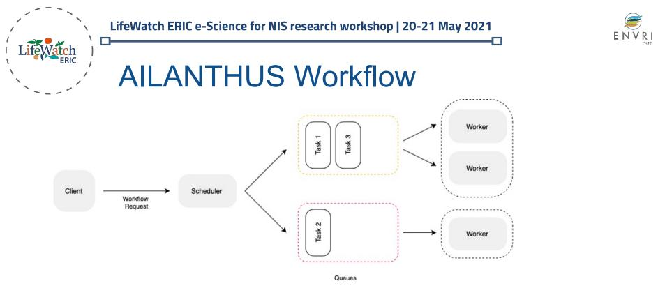
TITAN's scheduler manages the queues in order to control the number of task in a queue. In this case, we have configured TITAN for checking if the next task is "SVM-Classifier-2", which requires an enormous amount of RAM memory, and thus, that component is executed in exclusivity in a worker.
